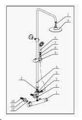
1.Shower valve X1 2.Washer X2 3.Diverter X1 4.Slider set X1 5.Handset holder X1 6.Hose nut X1 7.Washer X2 8.Handset X1 9.Head shower X1 10.Wall elbow X2 11.Cover plate X2 X2 12.Washer
